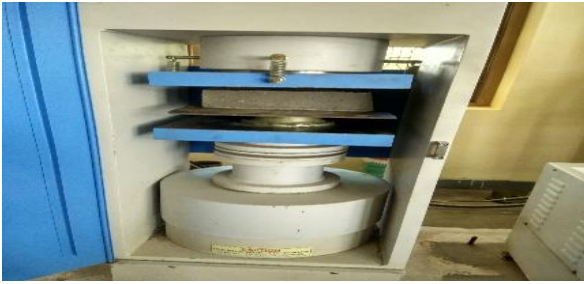
Figure 6 Crushing Strength of Fire Exit Brick
