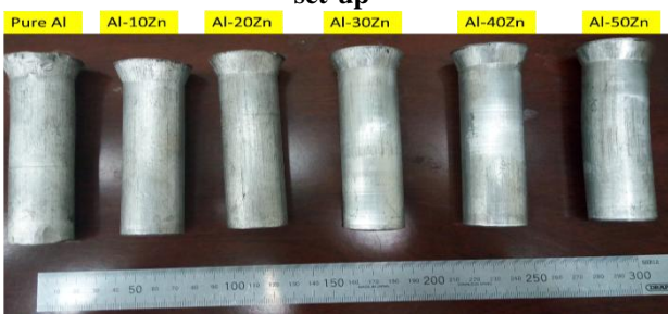
Figure 2. Photographs of Squeeze cast followed by extruded Al- xwt.% Zn castings
