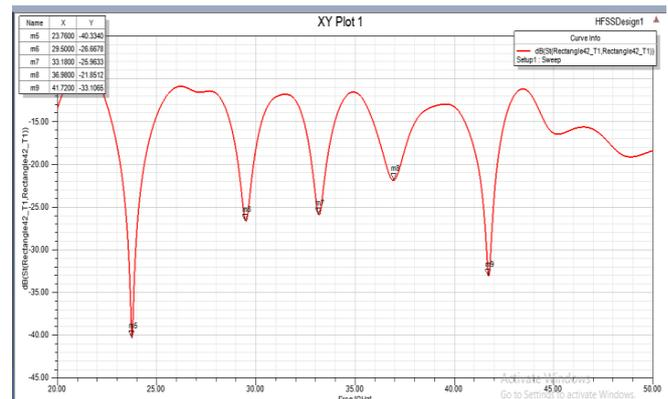
Fig 9. Return Loss for Base shape.
