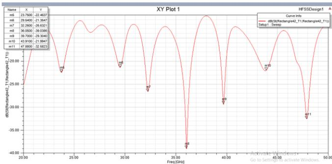
Fig 19: Return Loss for 2nd Iteration.
