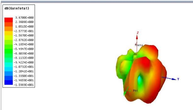
Fig 12. 3D gain for Base shape.
