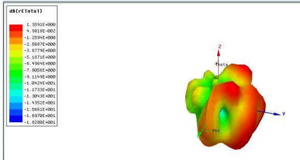
Fig 11. 3D Radiation Pattern for Base shape.
