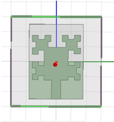
Fig 8: Second Iteration of Proposed Antenna
