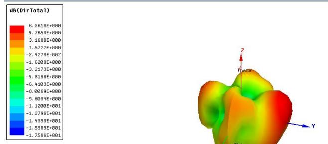
Fig 23: 3D Directivity for 2nd Iteration
