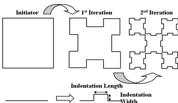
Fig 5: Iterative generation Procedure for a Minkowski Fractal
