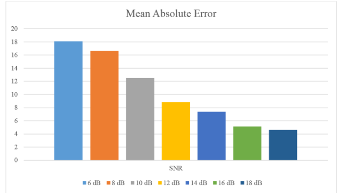
Figure 10: Bar graph for Mean Absolute Error calculation under different SNR (6-18 dB) in MIT-BIH data
