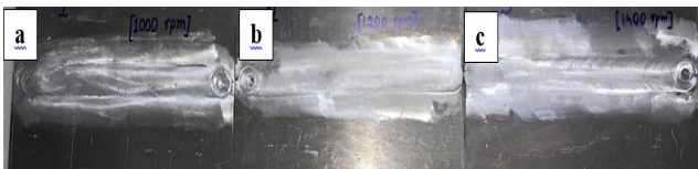
Fig. 3. 3(a) CTTP weldment at 1000 rpm 3 (b) CTTP weldment at 1200 rpm 3 (c) CTTP weldment at 1400 rpm
