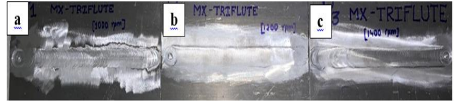
Fig. 6. 6(a) STFP weldment at 1000 rpm 6 (b) STFP weldment at 1200 rpm 6 (c) STFP weldment at 1400 rpm
