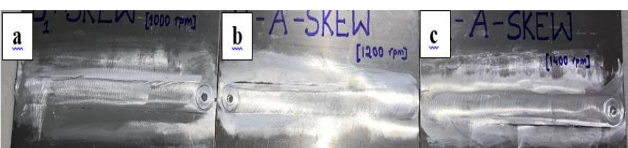
Fig 4. 4(a) IRAP weldment at 1000 rpm 4 (b) IRAP weldment at 1200 rpm 4 (c) IRAP weldment at 1400 rpm
