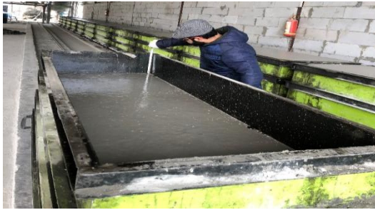
Figure-4: Analysis of aeration process of Autoclaved aerated concrete.
