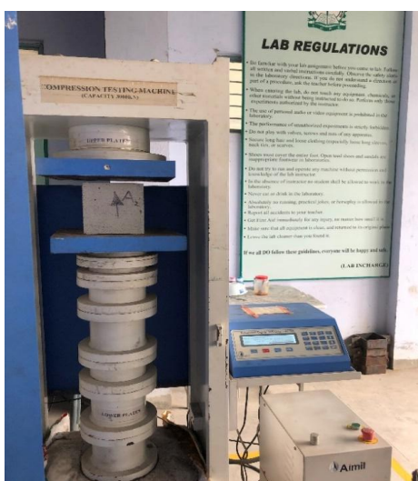
Figure-2: Compression test of the cube specimen of AAC.
