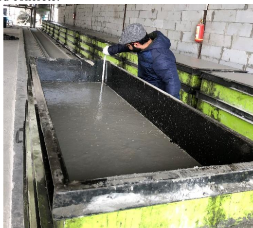
Figure-4: Analysis of aeration process of Autoclaved aerated concrete.
