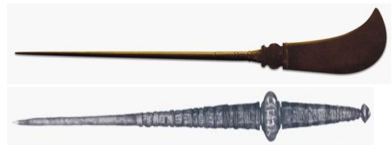
Fig.1 Types of metal stylus used for engraving [1]
