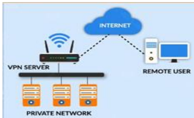
Fig. 3: Remote Access VPN
