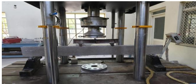
Fig.3 Four point bending test on reinforced beam
