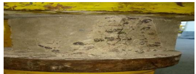
Fig.2 Two point loading test on concrete prism
