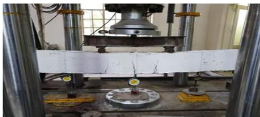
Fig 7. PCC Beam under Four-point load testing
