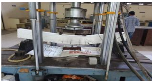
Fig 6. GPC Beam under Four-point load testing
