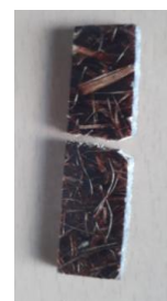
Fig.1(b). Sample after impact test
