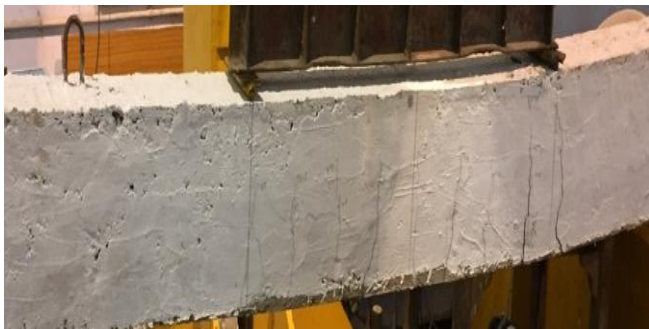
(b) Failure mode of RC beam with fibre (1.0%)
