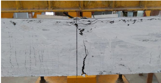
(a) Failure mode of reference beam (without fibre)
