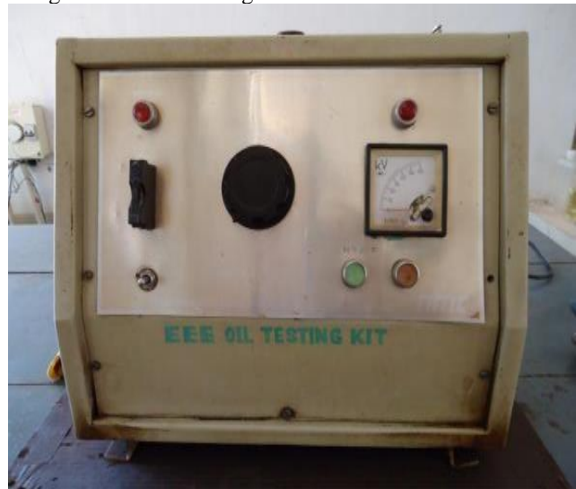
Fig. 7. Breakdown voltage kit - Setup
