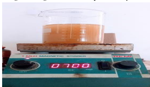
Fig. 2. Mixing of accelerate solution with vegetable oil
