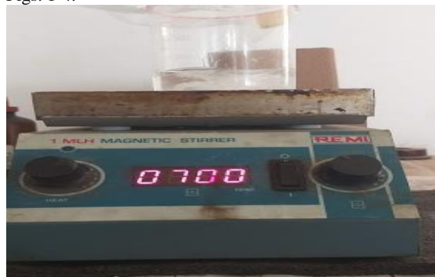
Fig. 1. Mixing of methanol and potassium hydroxide
