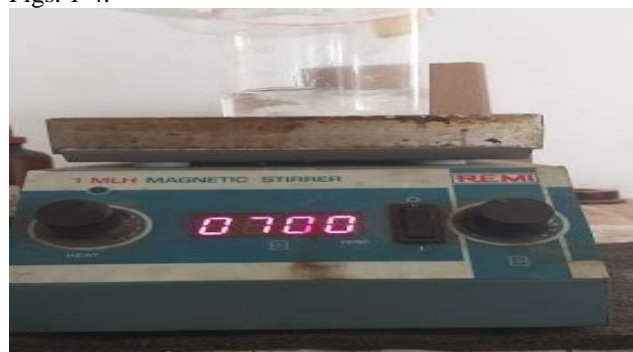
Fig. 1. Mixing of methanol and potassium hydroxide
