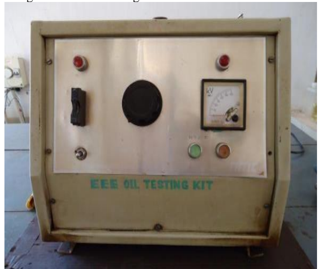
Fig. 7. Breakdown voltage kit - Setup
