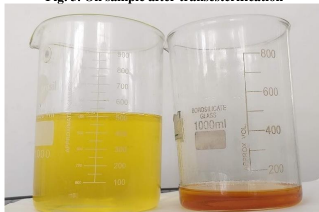
Fig. 4. Oil Sample after separation of ester and glycerol
