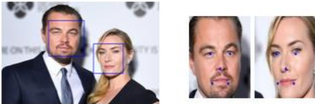
Fig. 5 : Bounding boxes found by a face detector, Aligned faces and point of reference.
