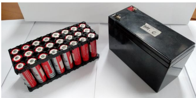
Fig. 4. Lithium-ion battery system and Lead-acid motorcycle battery
