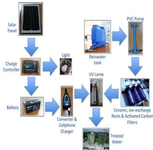
Fig. 1. Operation diagram of Water-Electricity-Light System
