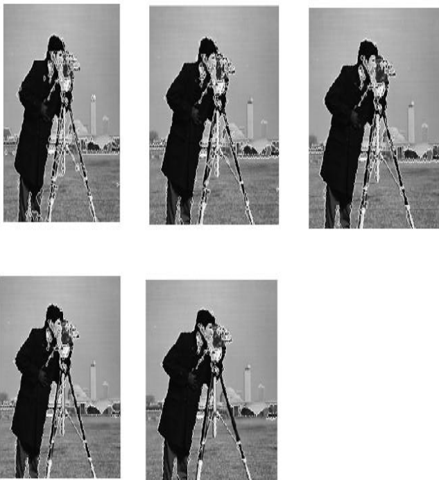
Fig 5: Clustered Cameraman image using Proposed Hybrid Clustering Algorithm with Clustering Radius 1 and different threshold values.
