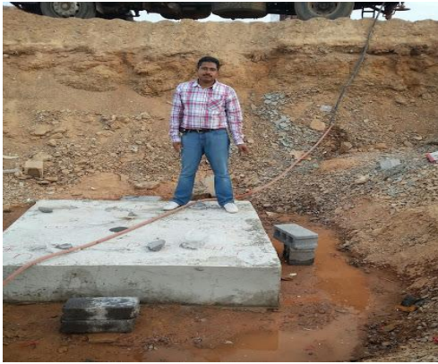
Fig. 7. Field footing model
