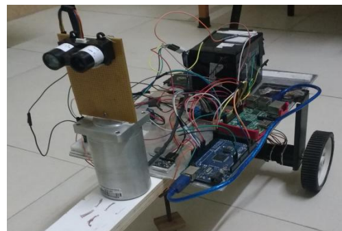
Figure 7: Hardware setup of the proposed obstacle detection and avoidance system
