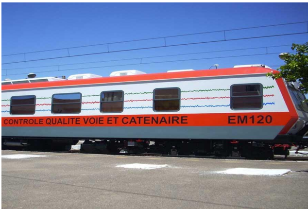
Fig. 3. Moroccan geometry measuring car EM120
