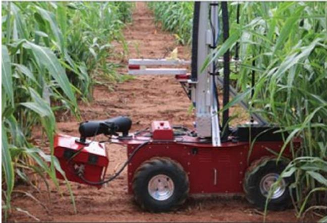
Figure 3: Custom stereo imaging sensor for stalks.
