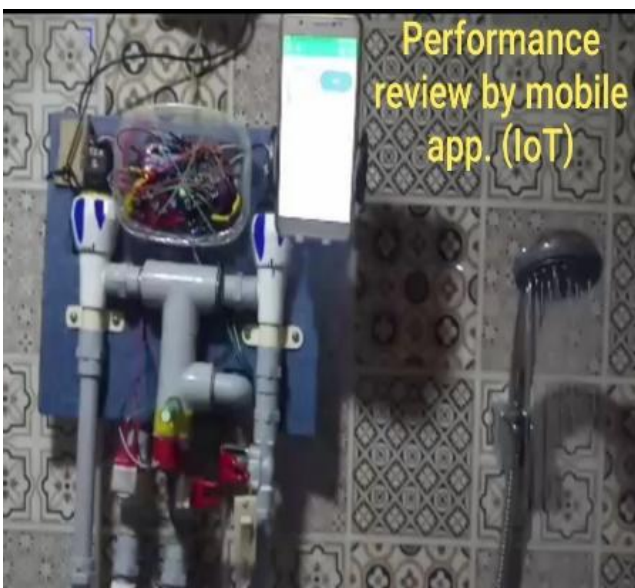
Figure: 3 IoT in a smart faucet
