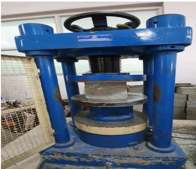
Figure 1 Test on concrete specimen
