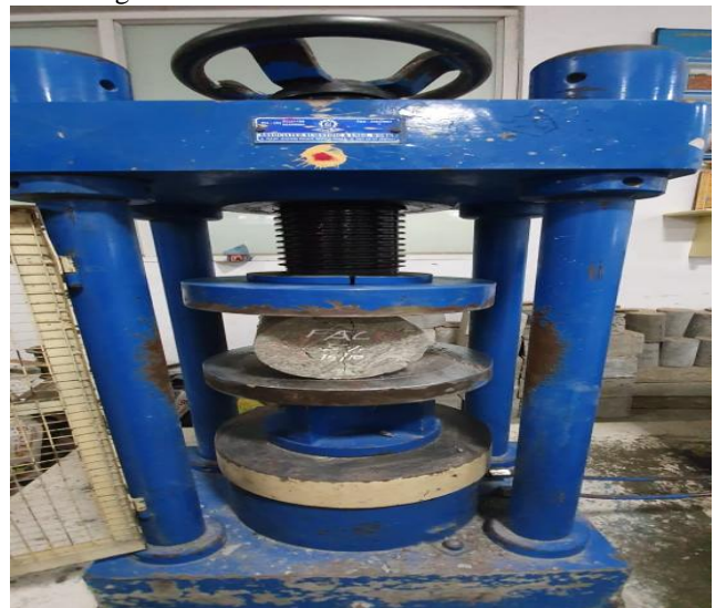
Figure 3 Test on cylindrical specimen
