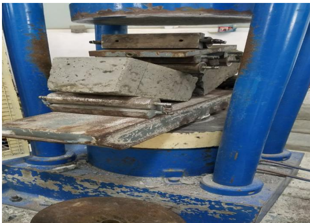
Figure 5 Test on prism specimen
