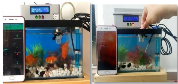
Figure 7. Testing of the turbidity sensor
