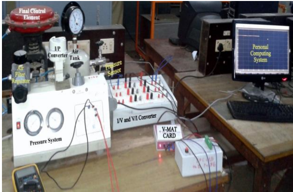
Fig. 2. Experimental setup of Air Pressure System (APS)
