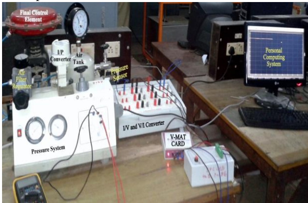
Fig. 2. Experimental setup of Air Pressure System (APS)
