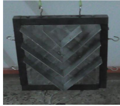
Figure 3. Plain Aluminium Plate with V-fins
