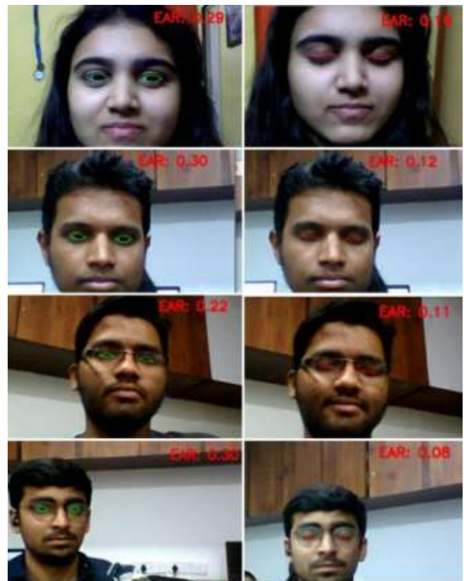
Figure 4. Model detects open and closed eyes based on the Eye Aspect Ratio
