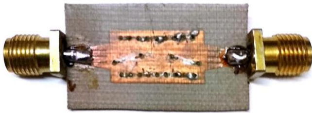
Fig. 5. Fabricated K-band Bandpass filter
