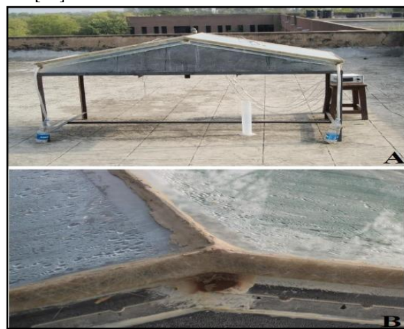
Fig. 1: (A) Pictorial diagram of solar distillation system (B) Mode of condensation
