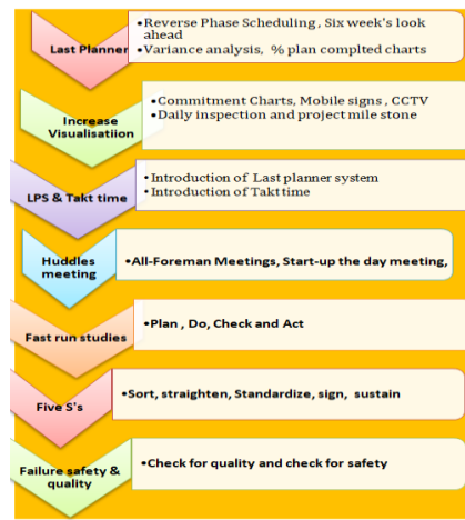
Fig 5: The implementation of the lean labour concept in Construction industry
