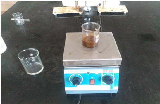
Fig.2 Preparation of nano Bio-Degradable cutting fluid
