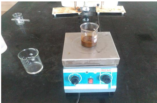
Fig.2 Preparation of nano Bio-Degradable cutting fluid
