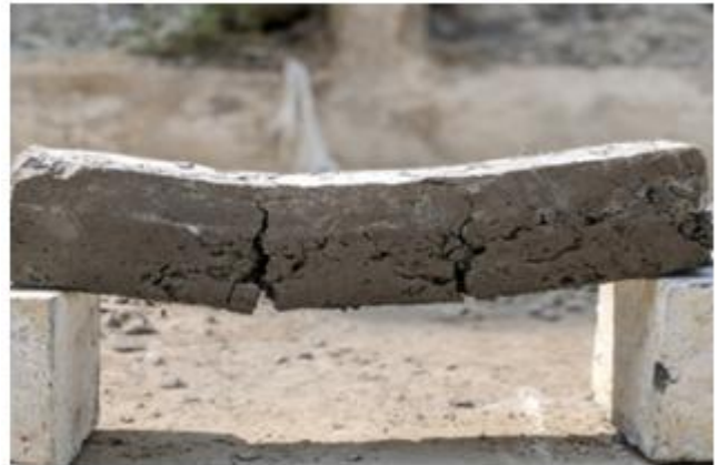
Fig.9 Bending in 0.1% of Rayon Fibre
