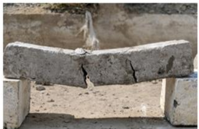
Fig.11 Bending in 0.2% of Rayon Fibre
