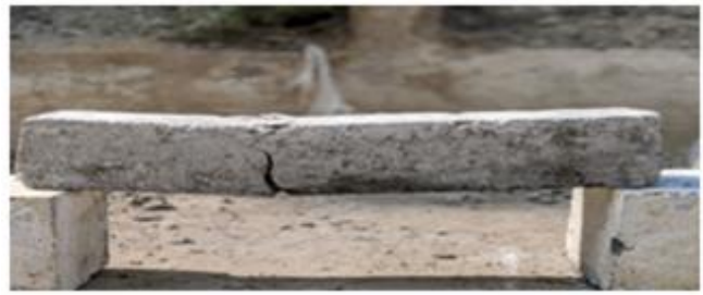
Fig.8 Bending in 0% of Rayon Fibre
