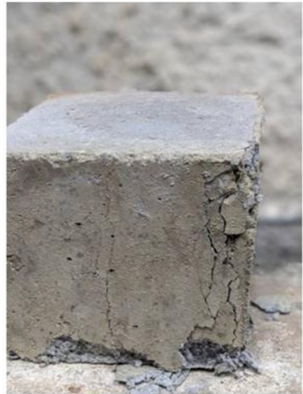
Fig.5 Failure in 0.1% Fibre Cube
