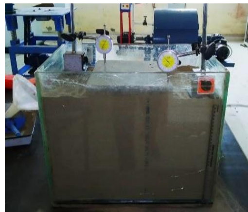
Fig 5 Testing of Pile Raft foundation
