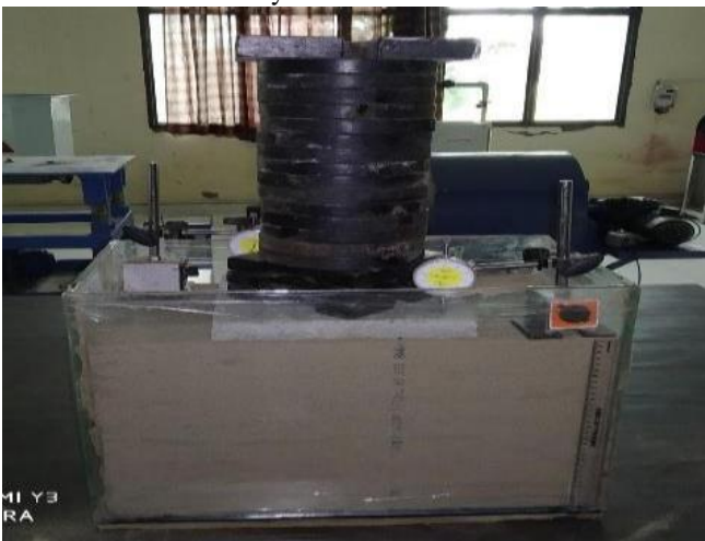
Fig 2 Testing of raft foundation
