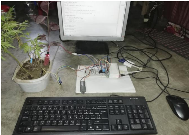
Fig10: Physical view of Smart Irrigation Monitoring & Controlling system in Agriculture
