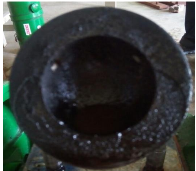
Fig.16.Piston head using diesel fuel
