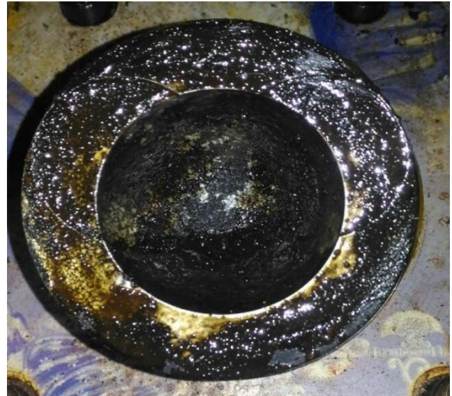
Fig.15.Piston head using B20 Blend
