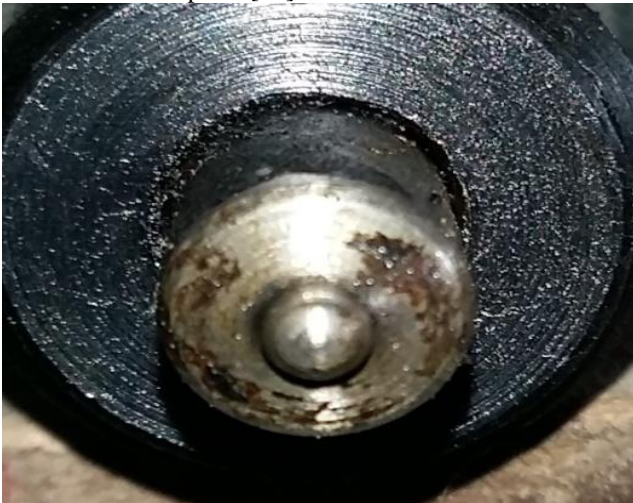
Fig.13.Injector using B20 Blend
