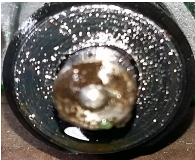
Fig.14.Injector using diesel fuel
