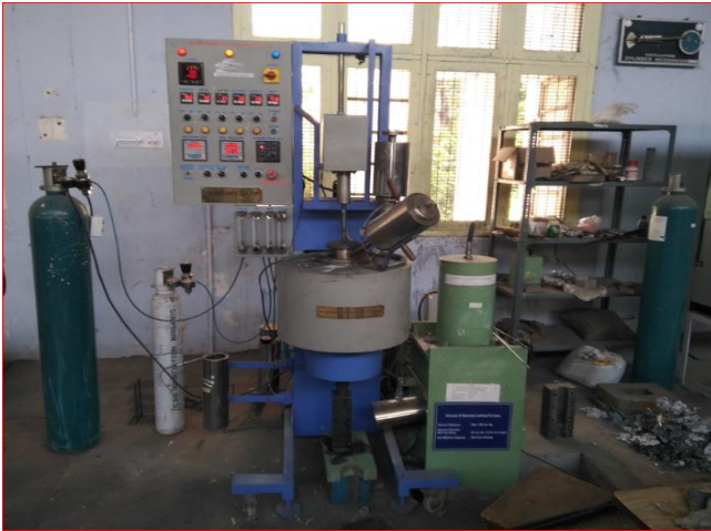
Fig 3.1.1 STIR CASTING SETUP
