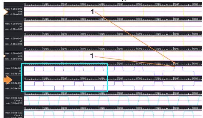
Fig.13 shows the simulation result of the control Logic Block(CLB) of the proposed system.
