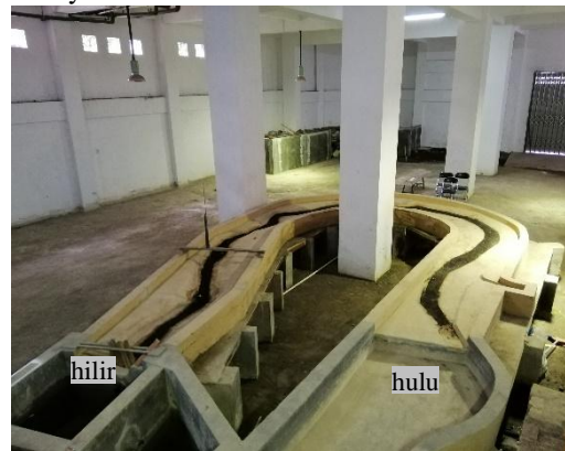
Fig. 2 Physical Model Test of Kahayan River
