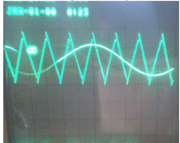
Fig. 10: Sinusoidal pulse with modulation with op amps.
