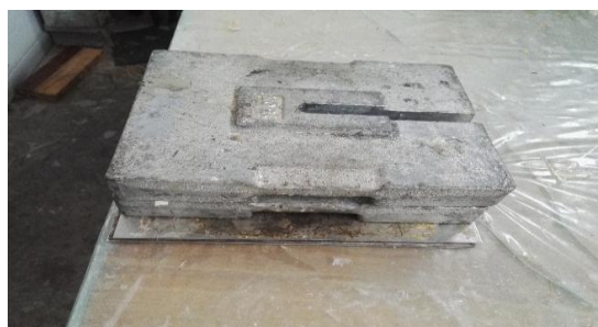
Fig. 1. Two 150 N load used in the experiment.
