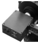
Fig. 7. SSP-7 Precision Photometer mounted on telescope.
