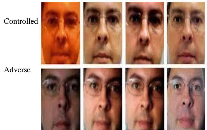
Fig. 4. Real faces and corresponding high definition, mobile and print attacks are shown from left to right[8]
