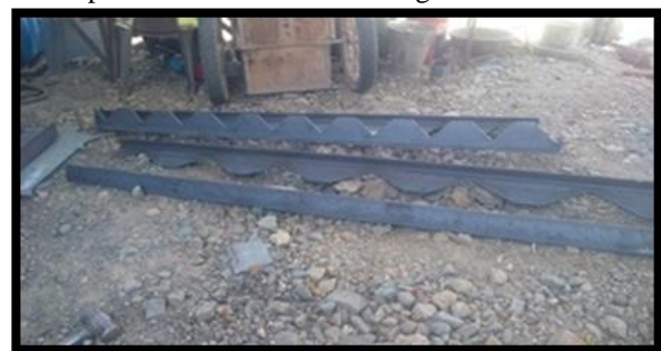
Fig. 6. Rearrangement of Castellated Beam
