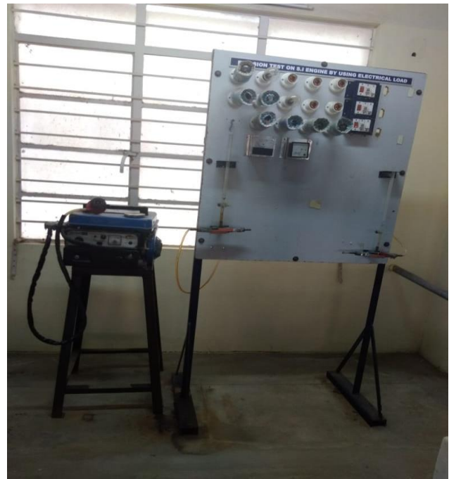
Figure 1 Single Cylinder 4 Stroke SI Engine Assembly with Electrical Load Test
