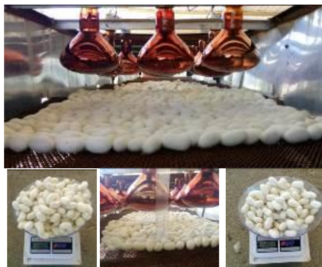
Fig. 4. The adjustment of the distance between the lamp and the cocoon in the process of dehydration of the living cocoon.
