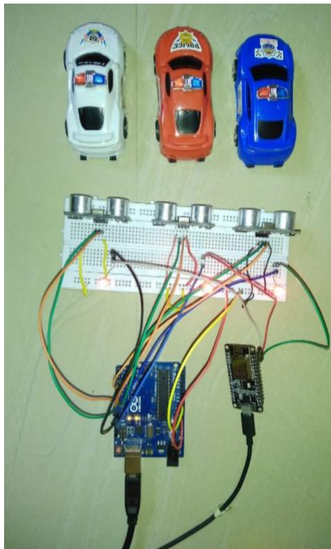
Figure5: Hardware connections of parking space 1
