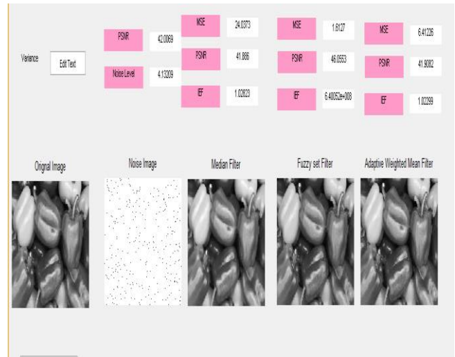
Figure 3 Comparison of Noise level & Median Filter ,Adaptive weighted filter and Adaptive Fuzzy Filter
