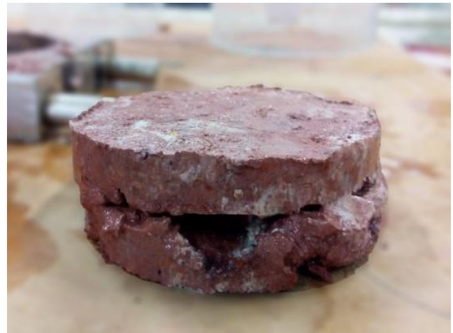
Fig. 11 : Loss of sample from fast shearing (0.05mm/min)
