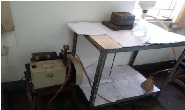
Fig 5. Pad formation vacuum pump
