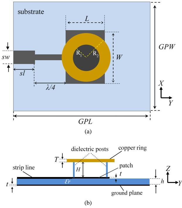
**Fig. 1. Schematic diagram of the QWT fed rectangular microstrip patch antenna. (a) Top view of a proposed MPA, (b) side view of a proposed MPA Parameters:  $GPL = 30.26$ ,  $GPW = 33.06$ ,  $W = 11.85$ ,  $L = 9.06$ ,  $sl = 5.3$ ,  $sw = 3.4$ ,  $R_1 = 3$ ,  $R_2 = 5.8$ ,  $\epsilon_r = 2.2$ ,  $h = 1.6$ ,  $t = 0.03$ ,  $H = 0.74$ ,  $T = 0.8$ , (all dimensions are in mm)**
