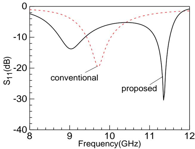
**Fig. 3. Comparison of simulated reflection coefficient characteristics of the antenna for with and without the metal ring. Parameters are same as in Fig. 1.**
