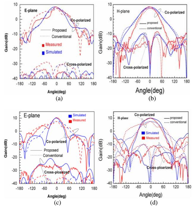
**Fig.7. Simulated and measured radiation characteristics of conventional and proposed MPA configurations, (a) E-plane, (b) H-plane radiations at 9 GHz, (c) E-plane, (d) H-plane radiations at 11.35 GHz. Parameters are same as in Fig. 1.**
