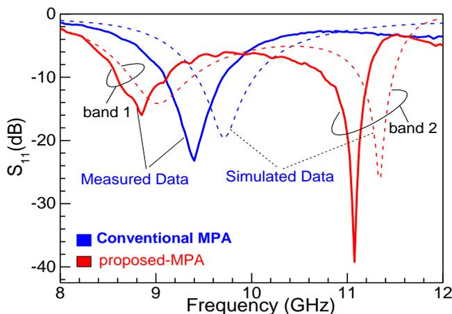
**Fig. 6. Simulated and measured  $S_{11}$  characteristics of conventional and proposed MPA configurations. Parameters are same as in Fig. 1.**
