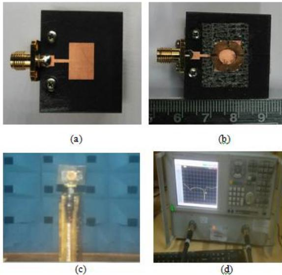
**Fig. 5. Antenna prototypes and the experimental setup: (a) top view of conventional antenna, (b) top view of the proposed antenna, (c) radiation pattern measurement setup in anechoic chamber (d)  $S_{11}$  measurement setup. Parameters are same as in Fig. 1.**
