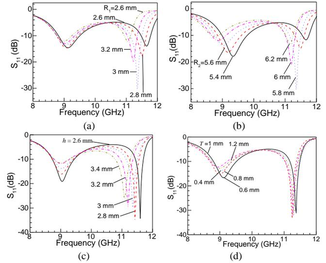
**Fig.2. Simulated  $S_{11}$  characteristics of the antenna due to the variation of metal-ring dimensions: (a) Inner radius ( $R_1$ ), (b) Outer radius ( $R_2$ ), (c) Height ( $H$ ), (d) Thickness ( $T$ ). Other parameters are as in Fig. 1.**
