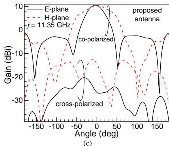
**Fig. 4. Simulated E- and H- plane radiation characteristics: (a) the conventional antenna at 9.7 GHz, (b) the proposed antenna at 9 GHz, and (c) the proposed antenna at 11.35 GHz. Parameters are same as in Fig. 1.**
