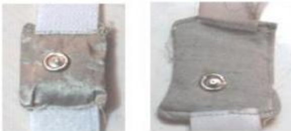
Fig. 3: Fabricated conductive textile electrodes (a) Type – I and (b) Type – II conductive fiber
