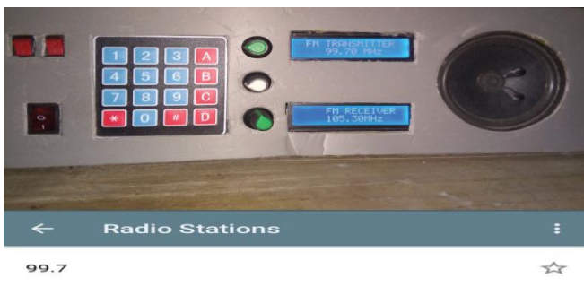
Fig. 13. Transmission channel at 99.7 MHz and reception channel at 105.3 MHz
