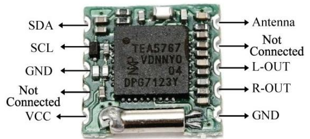
Fig. 5. Pin-out diagram of TEA5767 module
