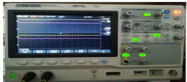
Fig. 15. Serial clock (SCL) and Serial data (SDA) signals
