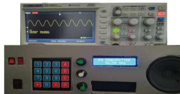
Fig. 16. Transmitted FM Signal at 96.50 MHz
